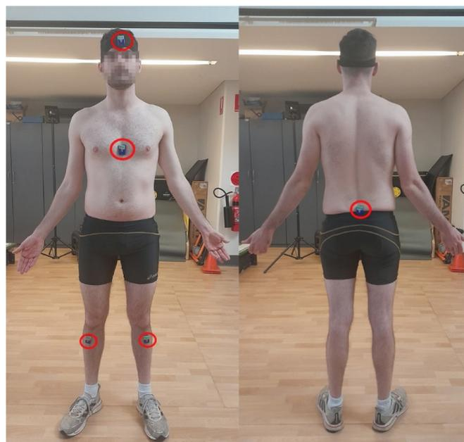
Figure 1. Placement of IMUs on the participant.
