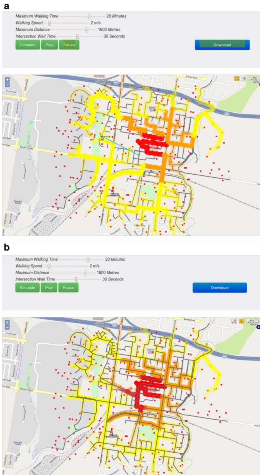
Figure 1 Screenshots showing the vector editing functionality of the simple agent-based modelling tool. a shows the vector addition in blue. b shows the agents traversing the new network.
