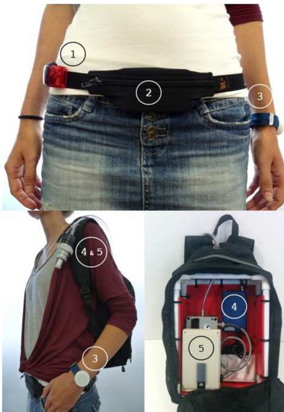
(1) ActiGraph wGT3X+; (2) Samsung Galaxy Young (GT-S5360) running ExpoApp; (3) Wrist Scienterra UV-B dosimeter; (4) MicroAeth Model AE51; (5) GK2.05 SH Cyclones and BGI/Mesa Labs 4004 Pumps (see details in Table S1).
