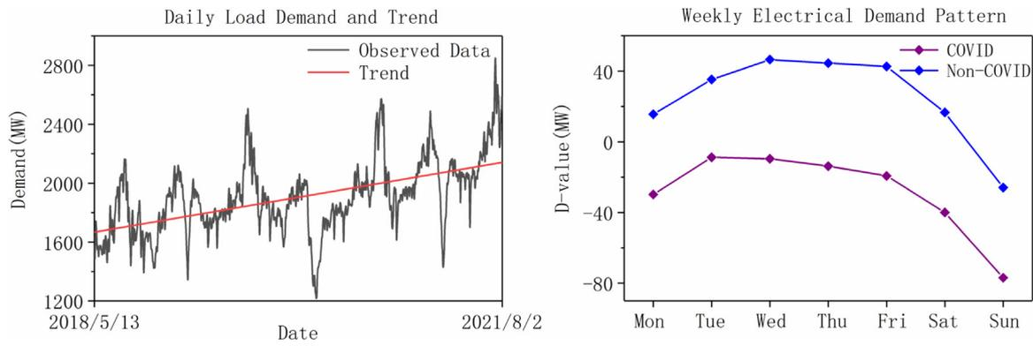
**Fig. 2.** Patterns for electricity demand. The left figure provides the daily demand and the trend. The right figure provides the comparisons between the COVID period and the non-COVID period where  $D\text{-value} = \text{Demand} - 0.4019\text{TimeOrder} - 1667$ .
