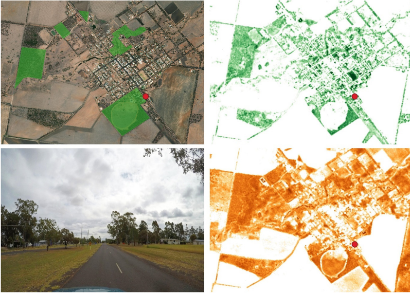
Figure 3: This panel shows (clockwise from top left). Queensland globe aerial image of Jandowae, Queensland with mapped nature conservation and recreation land uses in green, NDVI image from Sentinel 2 with index values shown as shades of green, fractional cover image from Sentinel 2, with vegetation cover shown as shades of brown and Mapillary streetview image taken at the location of the red point.
