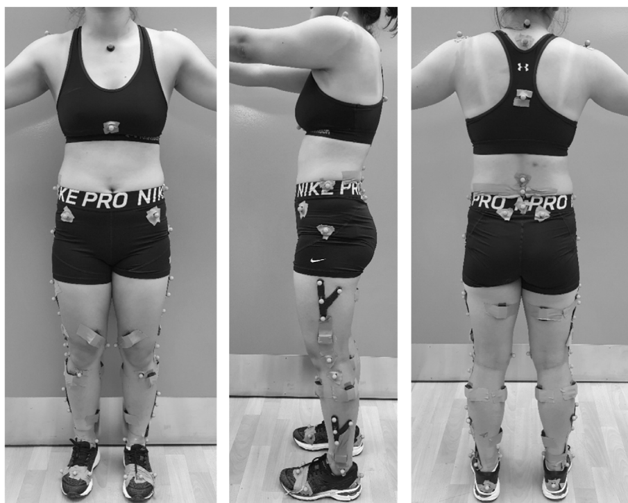
Fig. 2. Reflective marker and cluster (thigh & shank) placement based on 6DOF and IOR models.
