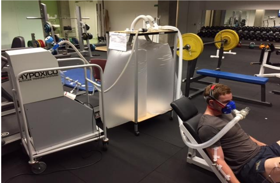
Figure 8. Hypoxic environment. The hypoxic generator was connected to a series of Douglas bags and further on the participant with the Hans Rudolf two-way valve facemask.
