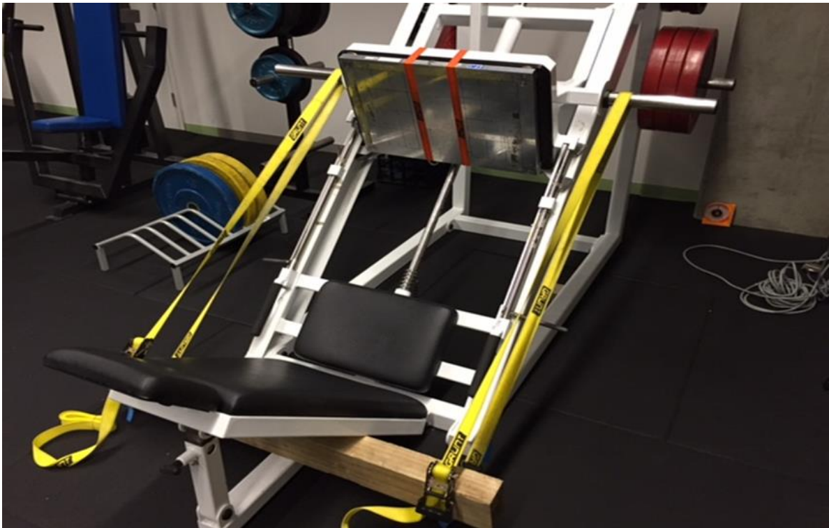
Figure 6. The customised leg press. The platform is locked in place by the ratchet tie down straps, so that the contraction is isometric. Each participant was seated at a knee angle of 60^\circ flexion when performing the MVC.
