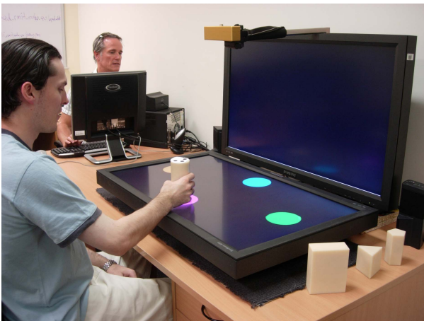
Fig. 2: Elements workstation for upper limb assessment. The Wii Sensor bar is mounted directly behind the stereo camera, from the user's perspective.
