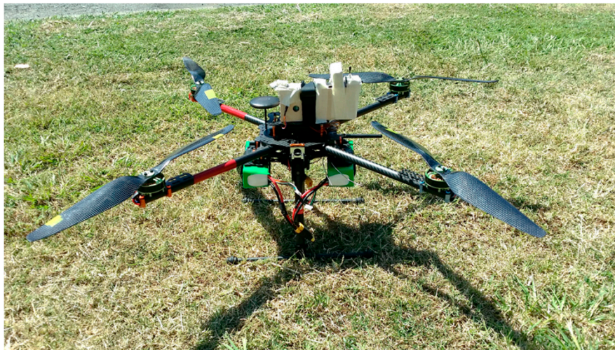
Figure 5. Quadcopter and modular gas-sensor system integrated.
