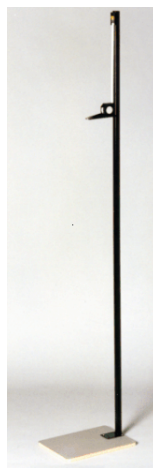
Figure 5.1: The portable stadiometer (Mentone Education Centre, Design number 1013522) used to measure stretch stature.
